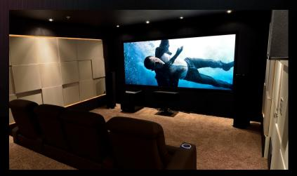
The Enlightor-4K fabric is held under permanent tension by a rigid aluminum frame that combines boldness in design, strength to span 300″ without sag. The 3.75″ wide frame is coated in our Infinite Black™ velvet which absorbs 99.7% of the incident light, creating the perfect black border.
