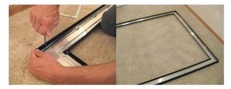
**Install Last Short Side.** For this fourth piece, a short side, insert its Lbrackets but do not tighten at this time. Align the four L-brackets into their mating slots into the top and bottom frame pieces and slide into position.
