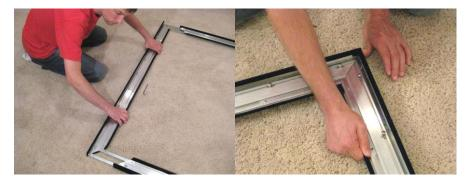
**Check Alignment, then Tighten Screws.** Confirming with your fingers that the joints are aligned nicely, go ahead and tighten the remaining set screws.
